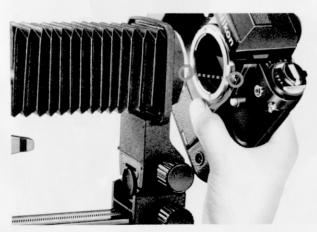
panel until it is positioned for vertical format photography. The motor drive-equipped camera can then be mounted in the usual way. Once the camera/motor drive combination is mounted, it can be turned to the horizontal position, if desired. Please remember that, whenever the camera/motor drive combination is rotated, the camera panel must always be racked all the way back to the end of the rail.
